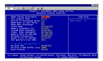
Figure 3.4: Advanced chipset features screen
